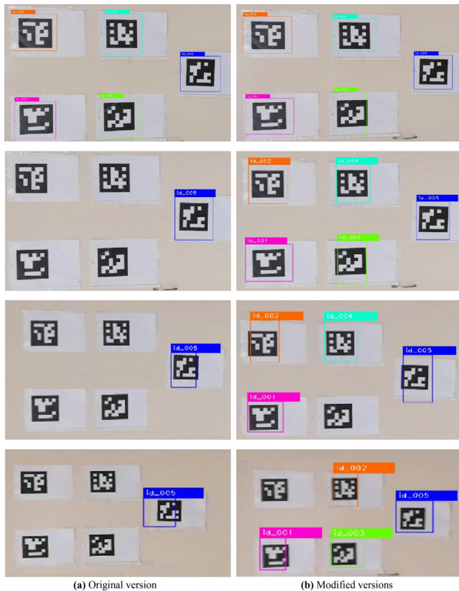
Fig. 19. Screenshots of detected markers from different distances (a) Original Tiny-YOLOv3 version (b) Modified Tiny-YOLOv3 versions.
